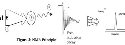
Figure 2: NMR Principle
